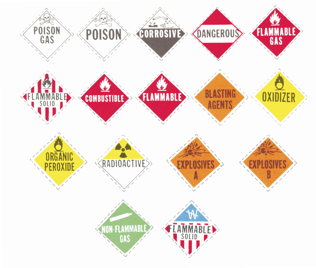
Figure 4-3.—Department of Transportation hazardous material shipping symbols.
